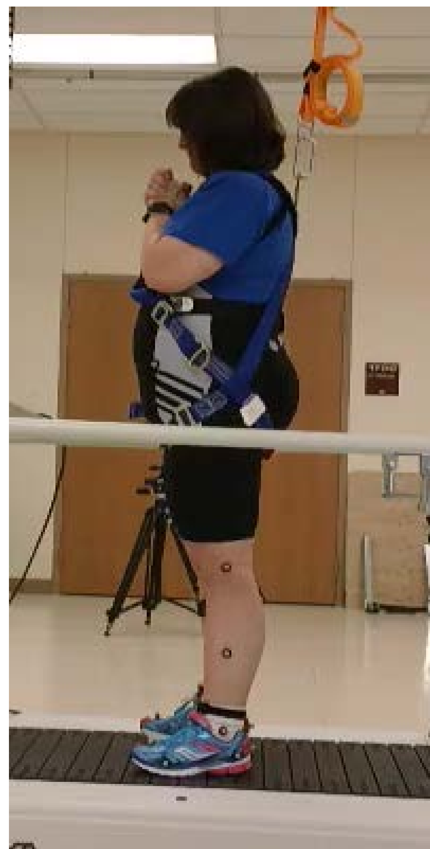
A subject prepares for a treadmill perturbation trial. The attached EMG sensors will identify the onset of activation of the TA and GN muscles.
