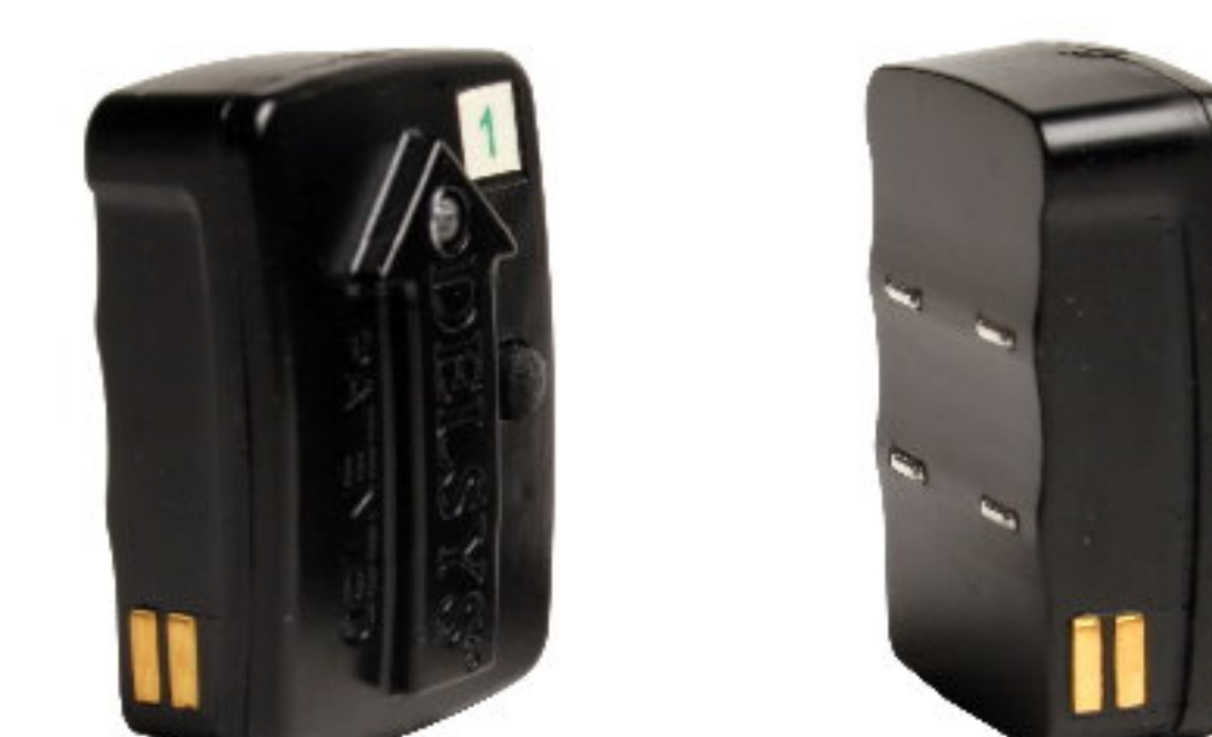
Front View Back View Delsys Trigno EMG sensors were affixed to the TA and GN muscles.
